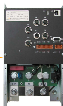
System Controller SC-3000 with Thyristor Module TS-3
